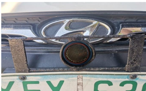
Figure 16. The ultrasonic sensor with metal bracket installed at the front bumper
