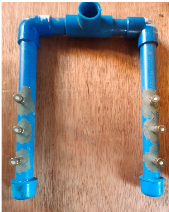
Fig. 1 4mm misting nozzle
