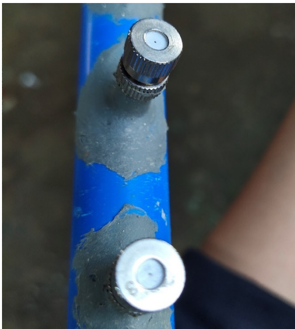
Fig. 2 3mm and 4mm misting nozzle
